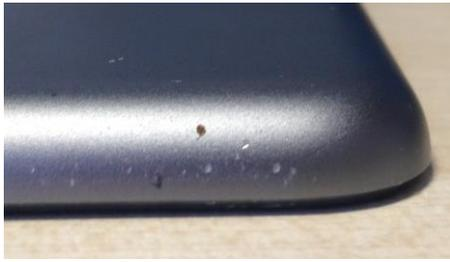
Case has been forced off using a pointed instrument leaving marks on the corner of the device.
